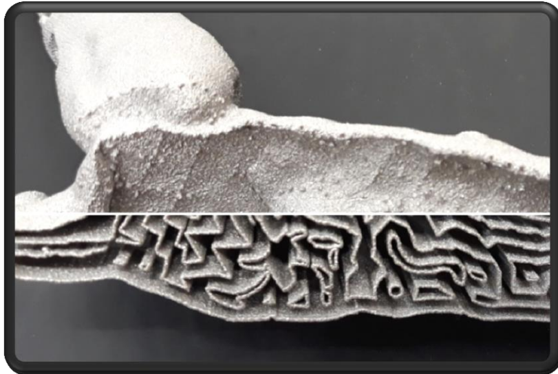
Removal of support structure
